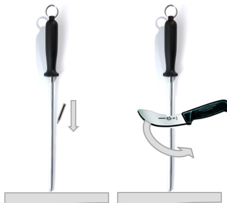
Figure 11: Sharpen a knife by holding the steel still and vertically on a flat stable surface
